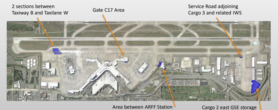
Distressed and damaged pavement areas to be replaced.
